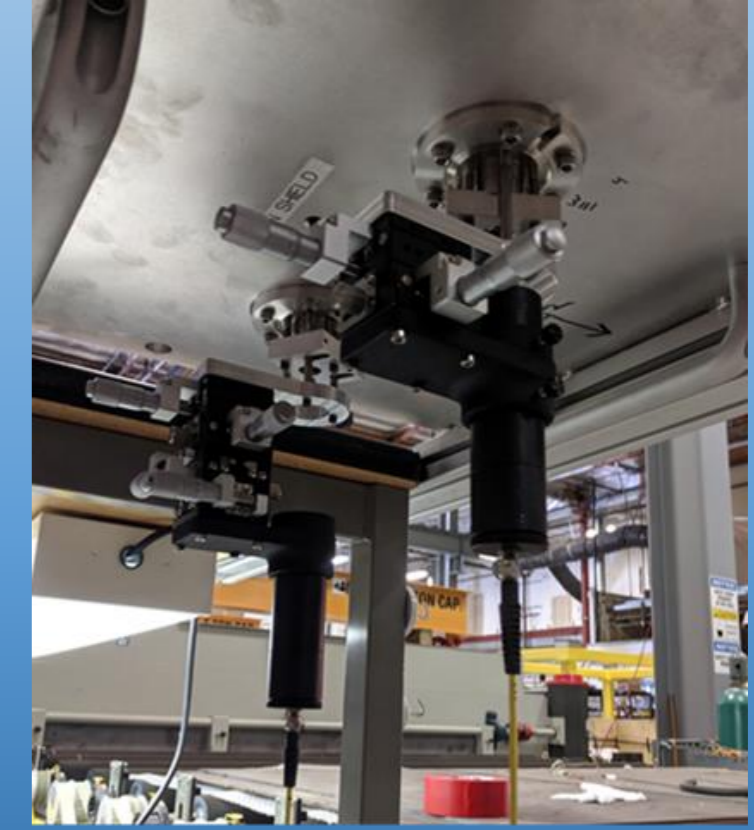
Periscopic Installation Outside Chamber
